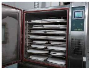
4. High and low temperature testing High temperature: 70 C Low temperature: minus 20 C
