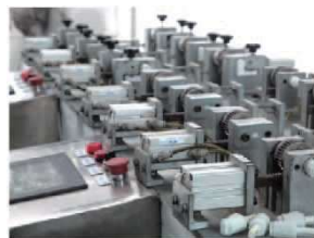
5. Damper intensity testing Resist 10000 cycles
