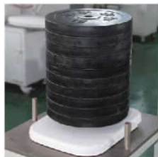
2. Static load testing Endure 150kgs load
