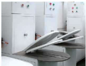
1. Life testing 60,000-100,000 cycle endurance
