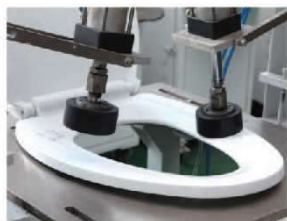
3. Sway testing Resist 25000 cycles of 1335N loading
